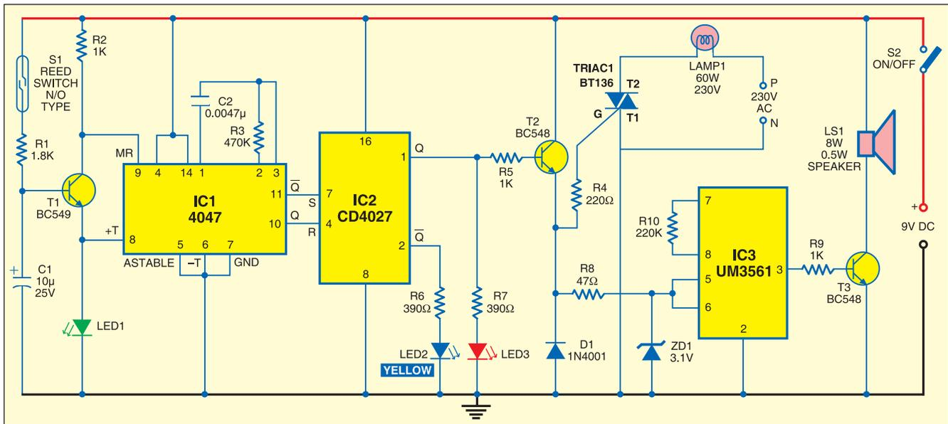
Fig. 1: Circuit of front door guard
