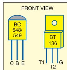
Fig. 2: Pin configuration of BC548/549 and BT136
