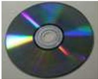
The CD weighs 15 – 20 grams and has a thickness of 1.2 mm. Its reflecting side is coated with a thin layer of Aluminium and protected with a layer of Lacquer. Standard CD has a diameter of 120 mm and can store 700 MB uncompressed data. This can run around 80 minutes. Mini CD and Digital Video CD are also available to suit the requirements of the user.
