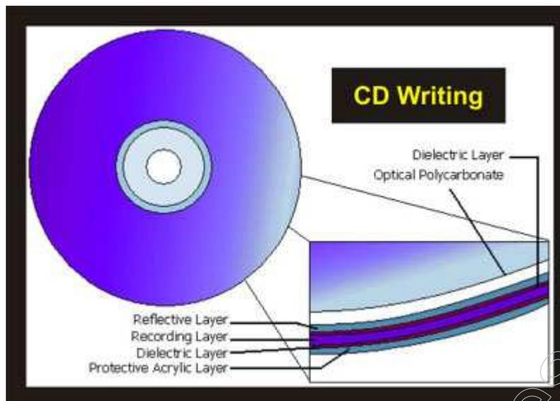
CD writer is used to burn the CD to record the data in the digital format. The CD burner darkens microscopic areas in the reflective side of the 'Blank CD'. During burning, both reflective and non reflective areas are created in the CD that can be interpreted as 1 and 0 by the CD player. The CD burner has a laser assembly similar to the CD reader. But the laser is 'Write Laser' with high power around 40 mW. The write laser interacts with the CD and alters its surface.
