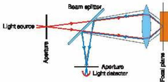
*Principle of Confocal microscopy*
