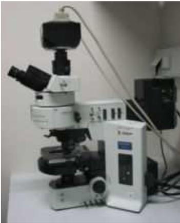
In fluorescence microscopy, the sample used to study is itself the light source. The technique is used to study specimens, which can be made to fluoresce. The fluorescence microscope is based on the phenomenon that certain material emits energy detectable as visible light when irradiated with the light of a specific wavelength. The sample can either be fluorescing in its natural form like chlorophyll and some minerals, or treated with fluorescing chemicals.
