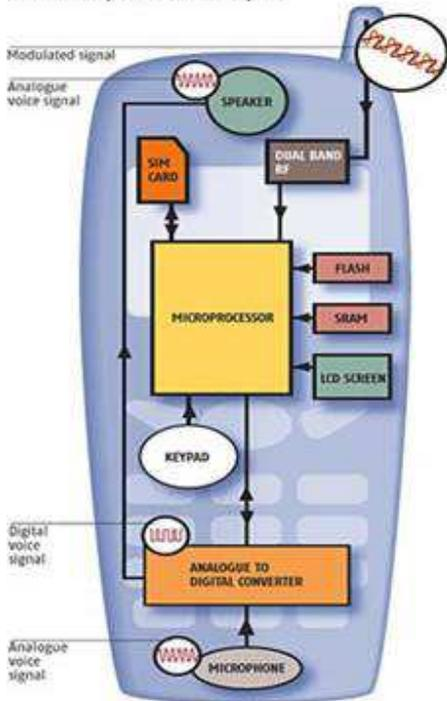
The circuit board is the heart of the Mobile phone. It has chips like **Analog-to-Digital and Digital-to-Analog** conversion chips that translate the outgoing audio signal from analog to digital and the incoming signal from digital back to analog. Following are the **Chips** present in Mobile phone.
