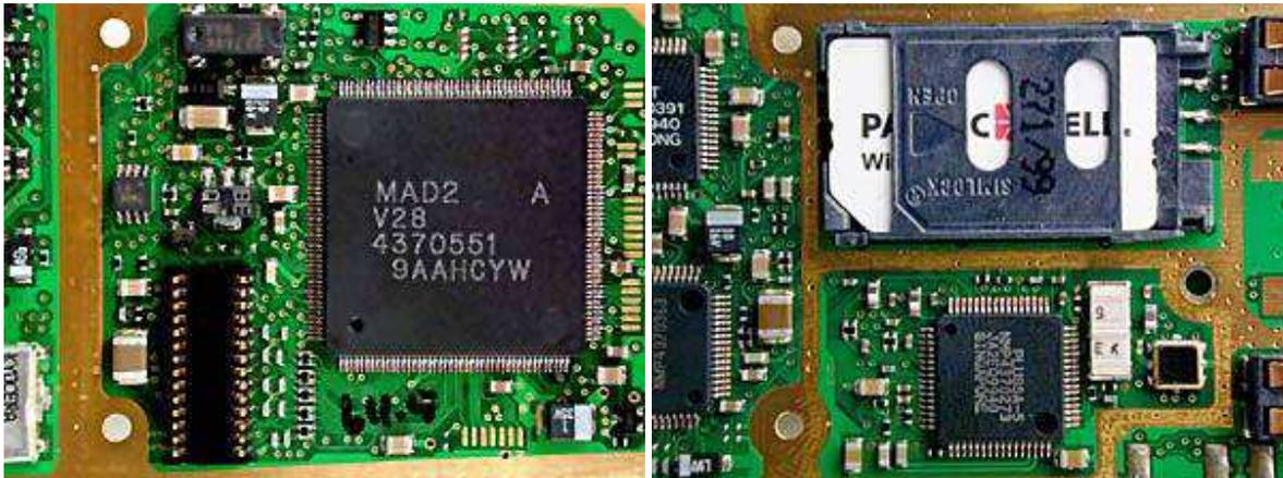
3. The Flash memory and ROM Chips of the Mobile phone act as a **storage location** for the phone. These chips store the customizable options of the cell phone, as well as the entire operating system. The power and radio frequency sections of the phone, phone recharging and power management etc are controlled by this chip. It also controls several hundred **FM channels**. The RF amplifiers focus on signals that go in and out of the phone's antennae.
